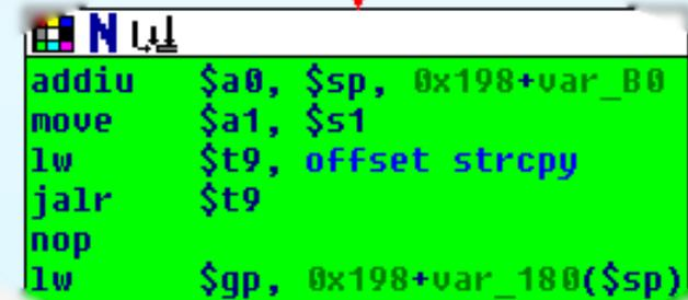
A screenshot of assembly code from a debugger. The code is displayed on a green background with a white border. A red arrow points from the top of the code block to the first instruction. The code includes instructions for adding an offset to the stack pointer, moving a register, loading a value from memory, jumping, and loading a global pointer.
