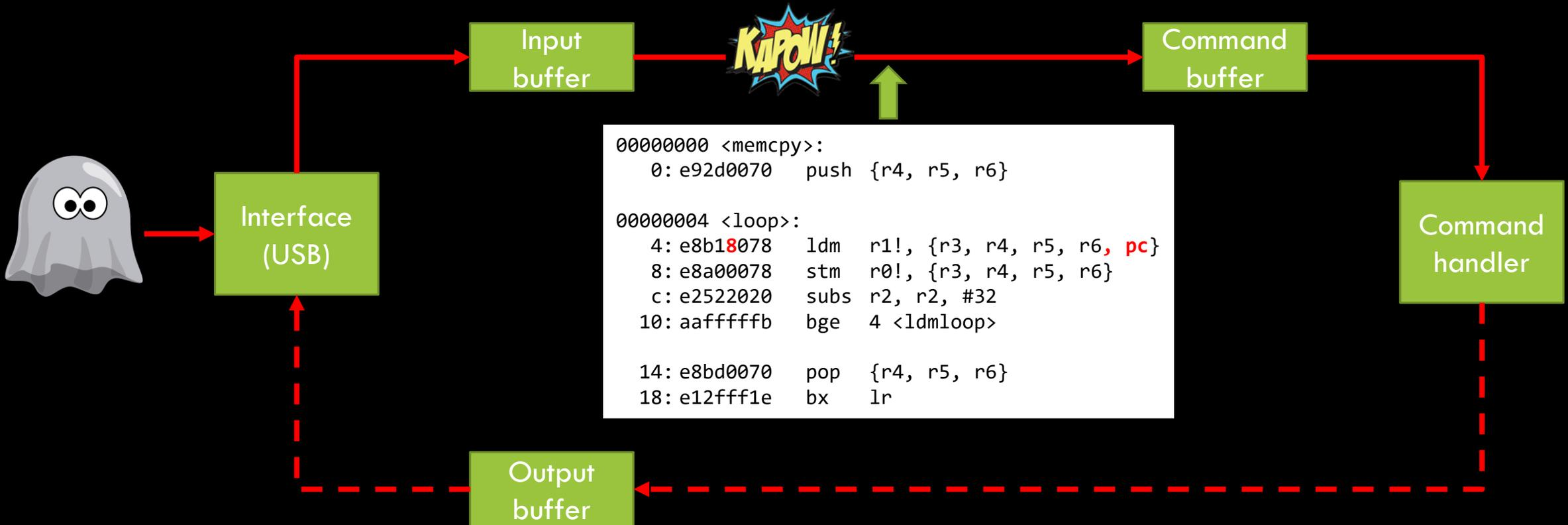
Control flow is **directly** hijacked using an 1 bit fault!
