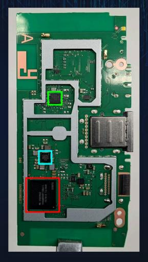
Note, the Quad-Core CPU in the SoC runs @ ~1.8 GHz !!!
